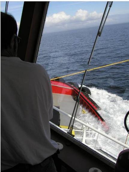
The captain switches the winch to Render / Recover mode to maintain constant line tension while positioning the tug to apply indirect steering forces on the tanker.
