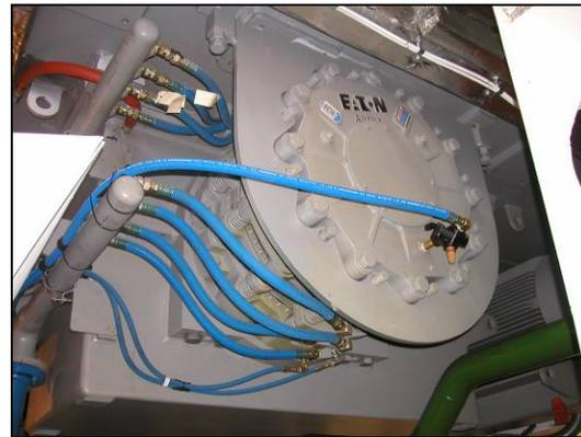
Water-cooled multi-disc slip brake
